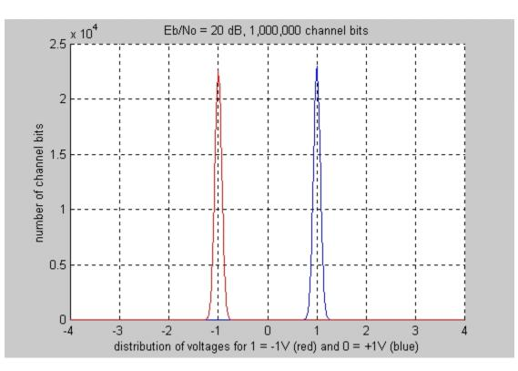
Transmission voltages (signal to noise ratio SNR 20 dB). No errors.
