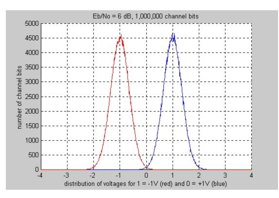
Transmission voltages with Gaussian noise (SNR 6dB) bit error rate (BER) of about 0.235%
